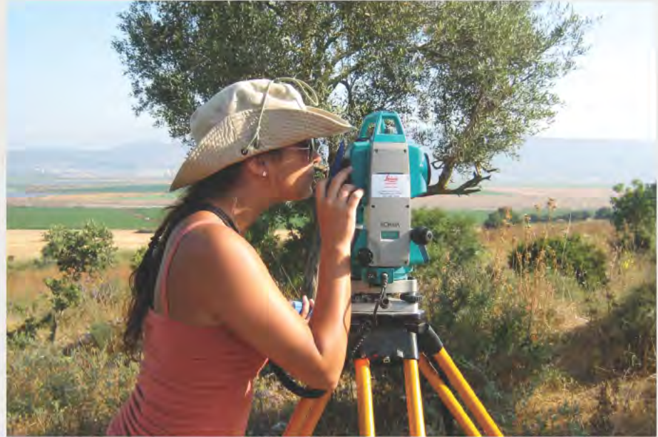
Samford student Erica Thornton uses the total station to survey a site in Israel.
